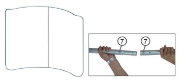
Connect all the pipes together according to the sticker number on each pipe. Make sure it is the same sticker number before you join the pipes.
