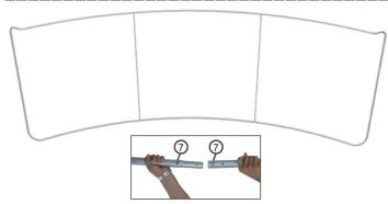
Connect all the pipes together according to the sticker number on each pipe. Make sure it is the same sticker number before you join the pipes.
